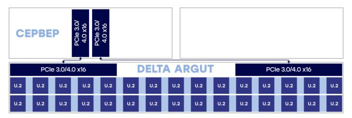
Standard advanced, up to 60 disks 1x Delta Tioga or Delta Serval 1x Delta Sprut 2x Delta Argut
